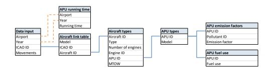
Figure 2: APU emissions and fuel use in the model
