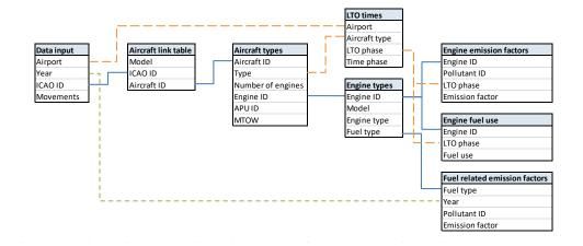
Figure 1: Aircraft LTO emissions and fuel use in the model
